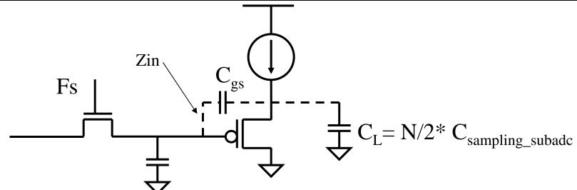
•  $C_L \alpha N/2$  sub-ADC caps, power/non-linearity increases as N increases for a given Sub-ADC speed to achieve high Fs.
