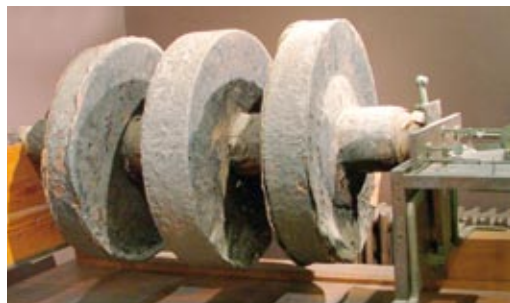
Callan's giant coil (1837) consists of three secondary coils connected in series on an iron core. Each coil contains about 10 miles of very fine wire insulated with a mixture of beeswax and gutta-percha. In 1837 this apparatus was able to produce sparks some 15 inches long.
