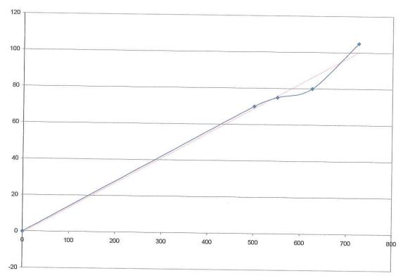
This ratio was later was put in place, when a specimen was placed on ground, and live parts were attached directly to the base. A calculated force was applied to blade, while readings were taken at switch bearing. The force was calculated based on NEMA SG-6 standard ( P=SV<sup>2</sup>, Where S is 0.0025 for cylindrical, and 0.004 for flat surfaces). The resulted data is pressure per square feet. These forces were them applied to a VM-1 motor operator.
