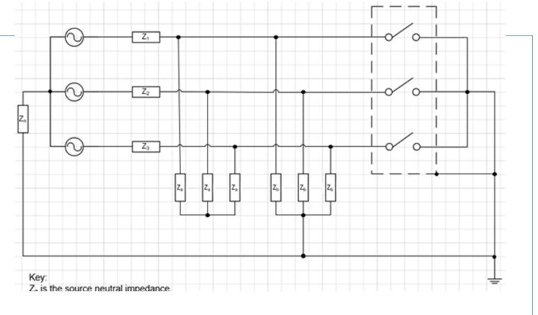
where  $Z_0$  zero sequence component of short-circuit impedance on supply side.
