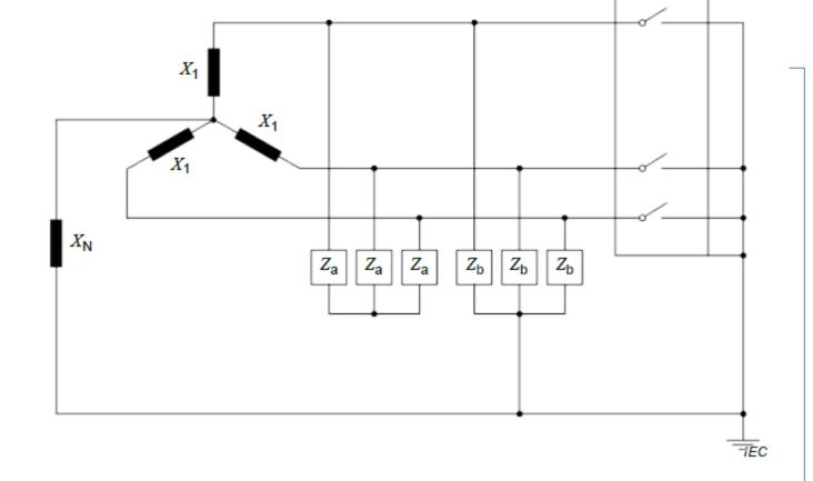
Figure 3 – Three-phase short-circuit representation
